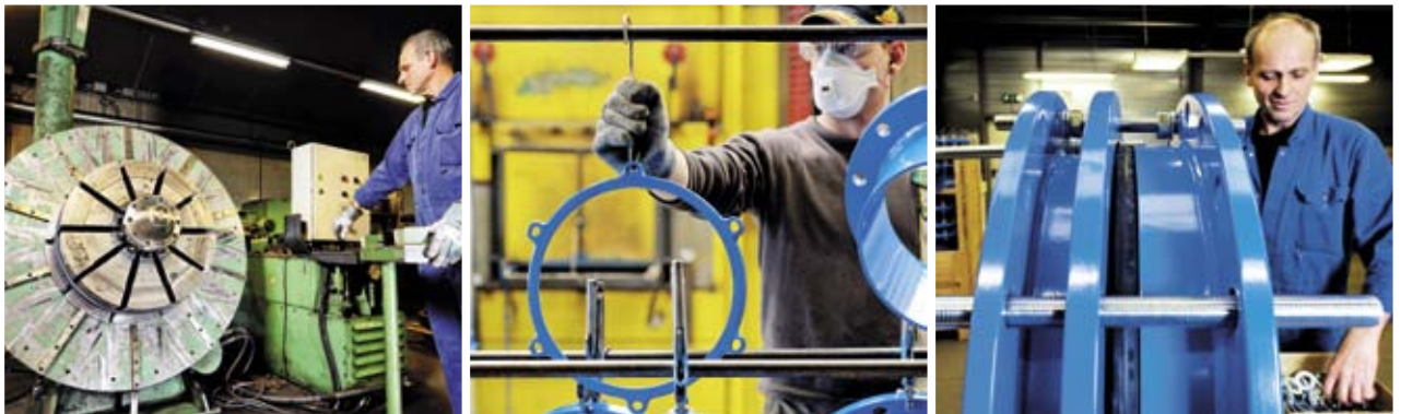
An expander guarantees an absolutely "round" product, the surface of which is protected by a high quality FBE coating. Subsequent steps are assembly and quality control.
