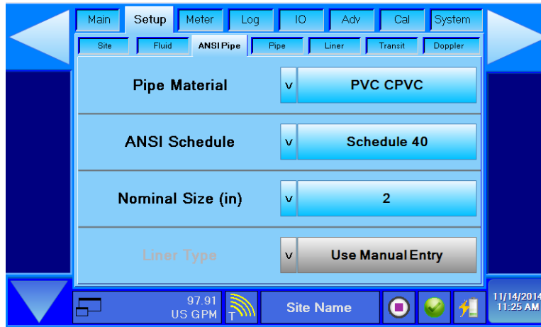
Figure 8: ANSI pipe setup
